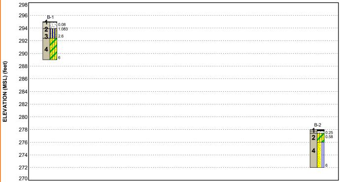
This is not a cross section. This is intended to display the Geotechnical Model only. See individual logs for more detailed conditions. Approximate boring elevations obtained from Google Earth.
