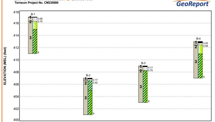
This is not a cross section. This is intended to display the Geotechnical Model only. See individual logs for more detailed conditions. Approximate boring elevations obtained from Google Earth.
